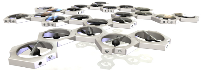
Fig. 1. This concept representation of the DFA is shown to be composed of a random arrangement of interconnected single-propeller modules that communicate with one another for coordinated flight.
