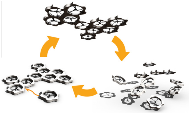
Fig. 1. This concept representation of the Distributed Flight Array (DFA) depicts the vehicle at different stages during its operating cycle. Starting from the lower left-hand corner of the figure, the modules assemble on the ground at random, generating a myriad of different possible network configurations. Once assembled, the modules coordinate and fly to a predetermined altitude and hover. After a certain amount of time, the modules break apart and fall back to the ground only to repeat the cycle in a new configuration.
