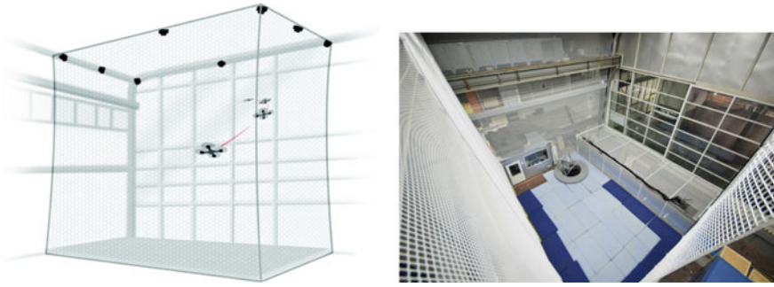
Fig. 4.3 The ETH flying machine arena. Left Schematic drawing showing the motion capture camera system that provides accurate measurements of the vehicle’s six degrees of freedom, position, and attitude. Right Photo of the installation at ETH Zurich. (Photo Raymond Oung)
